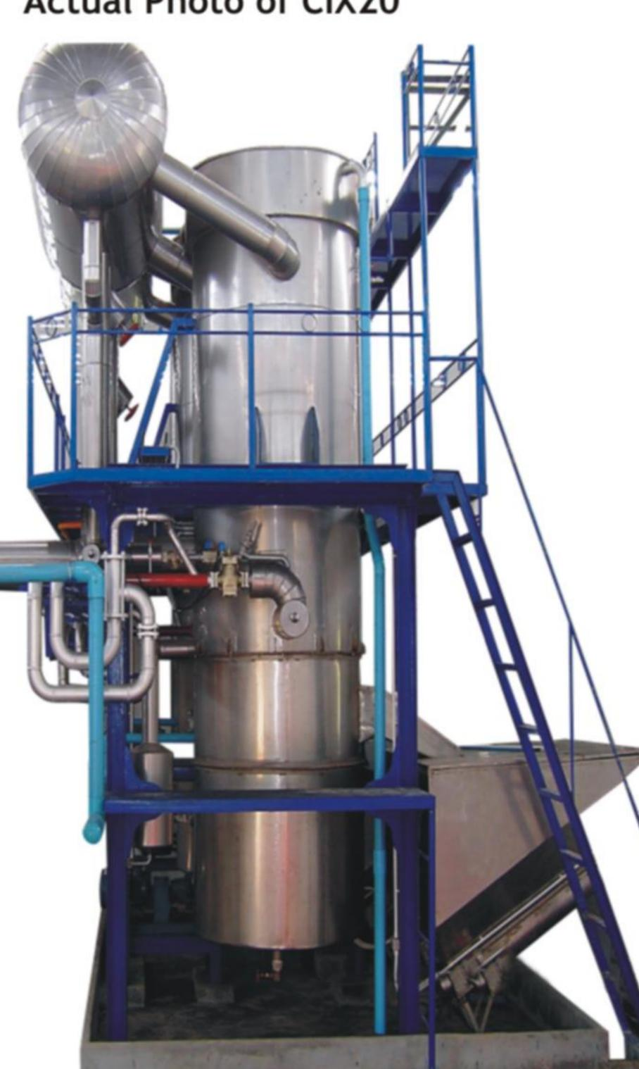
Metalex Tube Ice Machines are designed specifically to Freeze Ice automatically in vertical tubes, hot pressure gas thaws tubes and the ice is cut by specially designed cutter. All surfaces in contact with water or ice are of stainless steel or other rust - resistant materials. Heavy duty framing, automatic operation optional PLC and the best guarantee in the business makes Metalex TIX machines the FIRST CHOICE for perfect ice applications.
