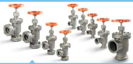
Fully fabricated valves, with replaceable teflon seats, available in flanged & direct welded options. Back seat arrangement possible (optional), for pressure up to 20 bar g & temperature range of -40  $^{\circ}$ C / + 120  $^{\circ}$ C. Sizes ½ inch (15 NB) to 6 inches (125 NB).
