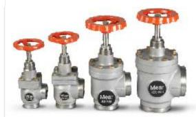
Cast steel construction, accepts flow In both directions. Can be used for most refrigerants including ammonia & non-corrosive gases. Available in "L" and "Y" type with direct welded options for pressure up to 20 bar g & temperature range of -40 °C to + 120 °C. Sizes available from ½ inch (15 NB) TO 6 inches (125 NB).
